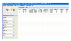
Six user-defined fields are available for custom data entry with each reading. Custom data can be exported with the weighing data.
